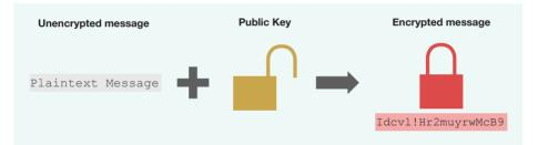
A message is encrypted with the public key, resulting in an encrypted message
